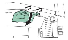
**3** Press in the tab on the right filter while removing it.
